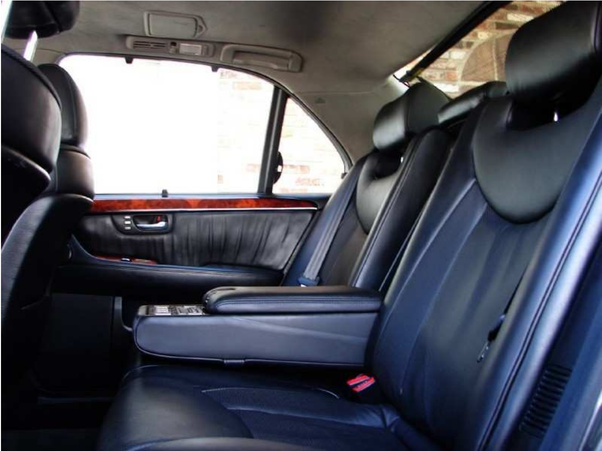
A/C vents above the rear doors (forward of the courtesy light) – UL only
