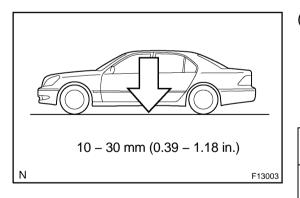
(d) With the vehicle in the HIGH position height adjustment, start the engine and change the height control switch from the HIGH position to the NORM position.
