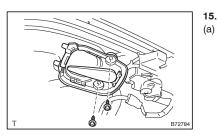
15. REMOVE LUGGAGE DOOR LOCK OPENER ASSY Remove the 2 screws and opener.
