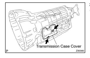
(b) Remove the refill plug and overflow plug.
