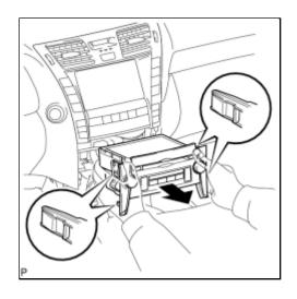
(b) Pull the radio receiver to detach the 4 clips on the backside of the radio receiver.
