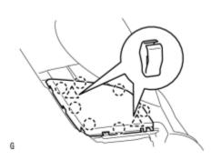
6. REMOVE NO. 1 INSTRUMENT PANEL SPEAKER PANEL SUB-ASSEMBLY
