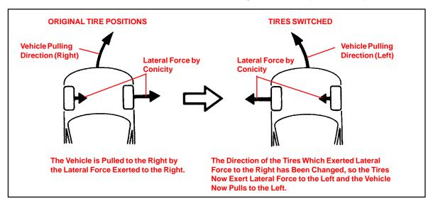
If the pulling direction does not change after the front tires are switched, the cause of vehicle pulling is not tire conicity. In this case, the likely cause is a front wheel alignment condition.
