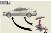
Turn the tire jack portion "A" by hand until the notch of the jack is in contact with the jack point.
