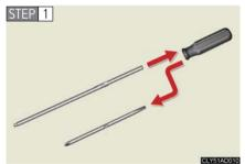
Take out the parking brake release tool and the screwdriver from the trunk. ( $\rightarrow$ P. 642)
