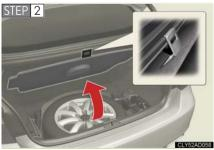
Secure the panel using the hook provided.
