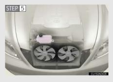
After the engine has cooled down, check the engine coolant level and inspect the cooling system for leaks.
