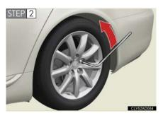
Slightly loosen the wheel nuts (one turn).
