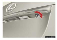
Turn the mechanical key clockwise to open.
