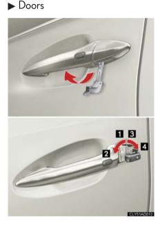
Remove the cover on the driver's door handle using the mechanical key in order to perform the following operations.
