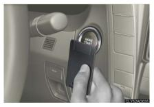
STEP 3 To change "ENGINE START STOP" switch modes: Within 5 seconds of the buzzer sounding, release the brake pedal and press the "ENGINE START STOP" switch. Modes can be changed each time the switch is pressed. (→P. 147)
