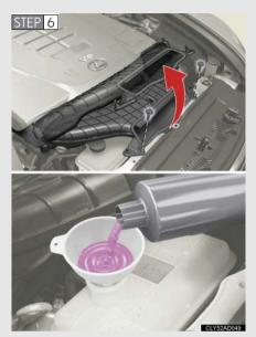
Add engine coolant if necessary.
