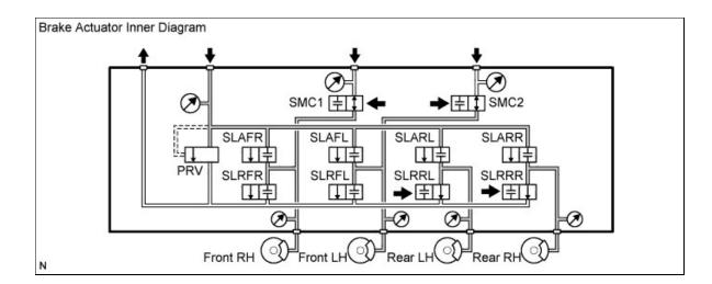
f. Check that each wheel cylinder's output value does not increase.
