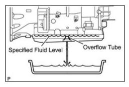
(k) Install a new gasket and the overflow plug.
