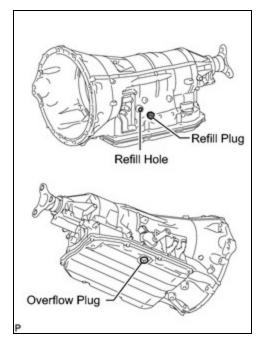
If the ATF flows from the overflow tube and the ATF flows in a thin stream, the fluid amount is normal.
