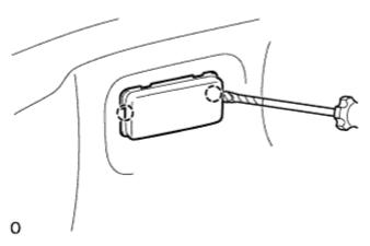
1. Using a screwdriver, detach the 2 claws and remove the light assembly. HINT:
