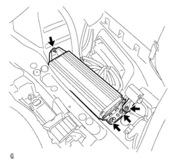
2. Remove the 4 nuts and amplifier with bracket.
