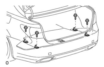
1. Remove the 4 bolts and 4 rope hooks.
