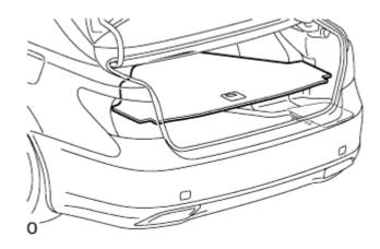
2. REMOVE BATTERY SERVICE HOLE COVER LH
