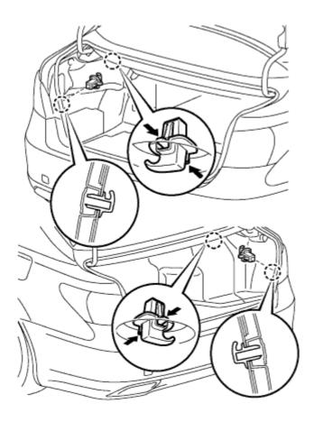
1. Remove the 4 rope hooks by pushing the claws in the direction of the arrows in the illustration.
