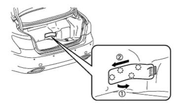
1. Pull the battery service hole cover in the direction of arrow 1, then slide it in the direction of arrow 2 to remove it.
