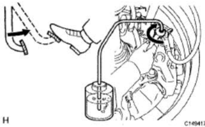
Fig. 8: Tightening Bleeder Plug And Release Brake Pedal Courtesy of TOYOTA MOTOR SALES, U.S.A., INC.
