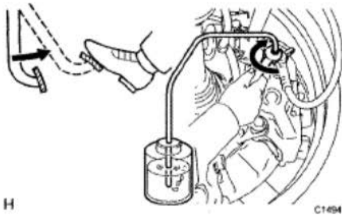
Fig. 16: Tightening Bleeder Plug And Release Brake Pedal Courtesy of TOYOTA MOTOR SALES, U.S.A., INC.
