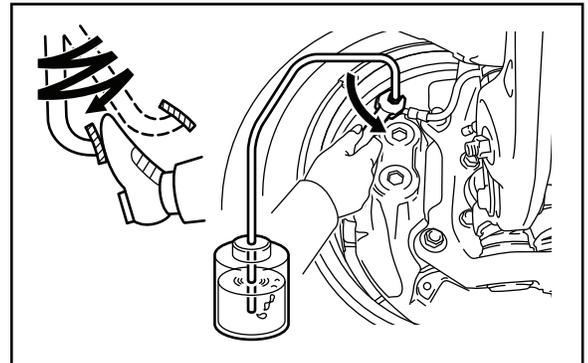
2. Pump and hold pressure on the brake pedal while an assistant opens the bleeder screw.
