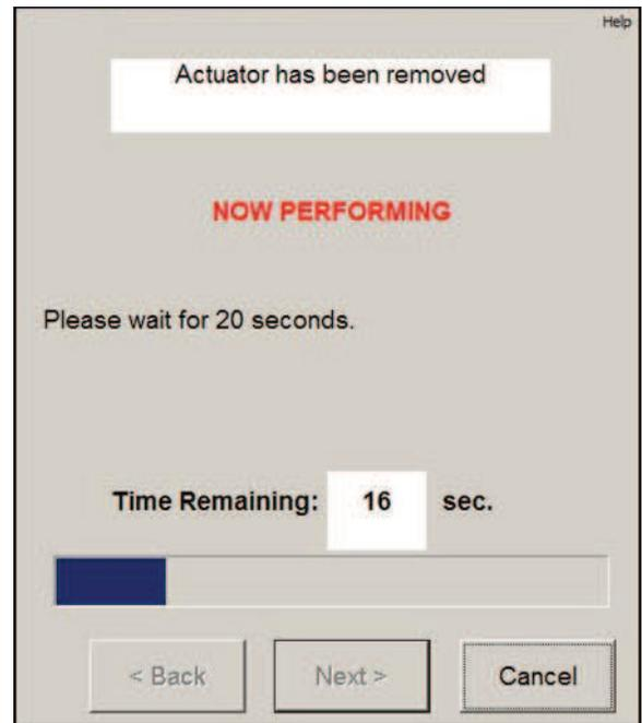
20. Press "Next" after cycling the ignition switch OFF and then ON. Press "Next" AFTER the pump motor stops running.
