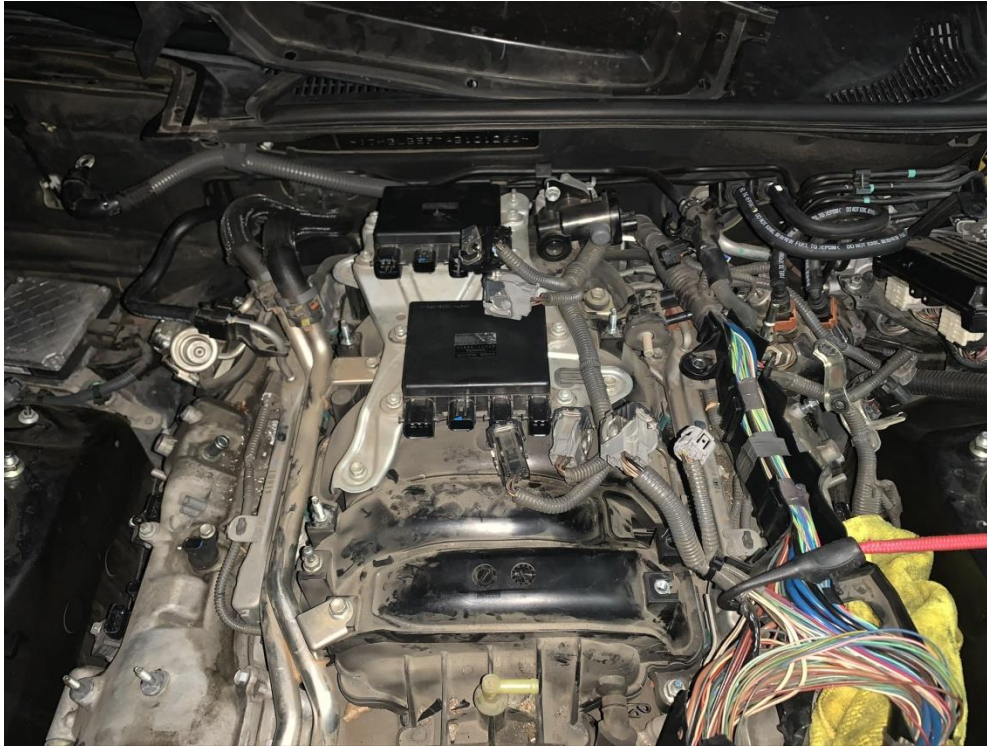
Removing the top electrical harness.
