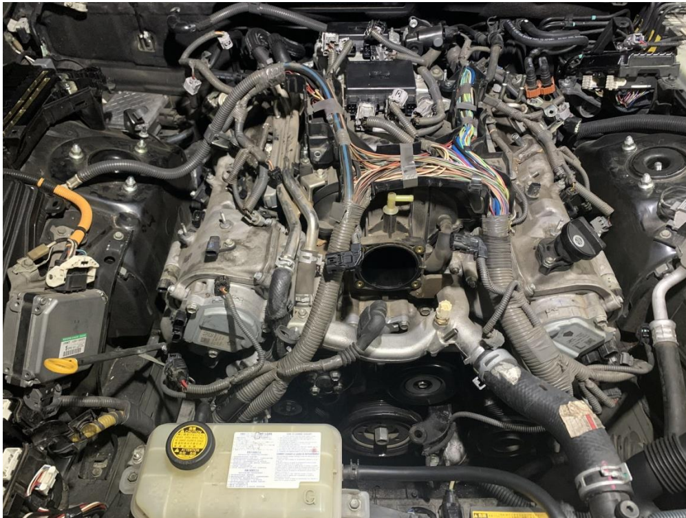
Removing the throttle body (which is optional – I think)
