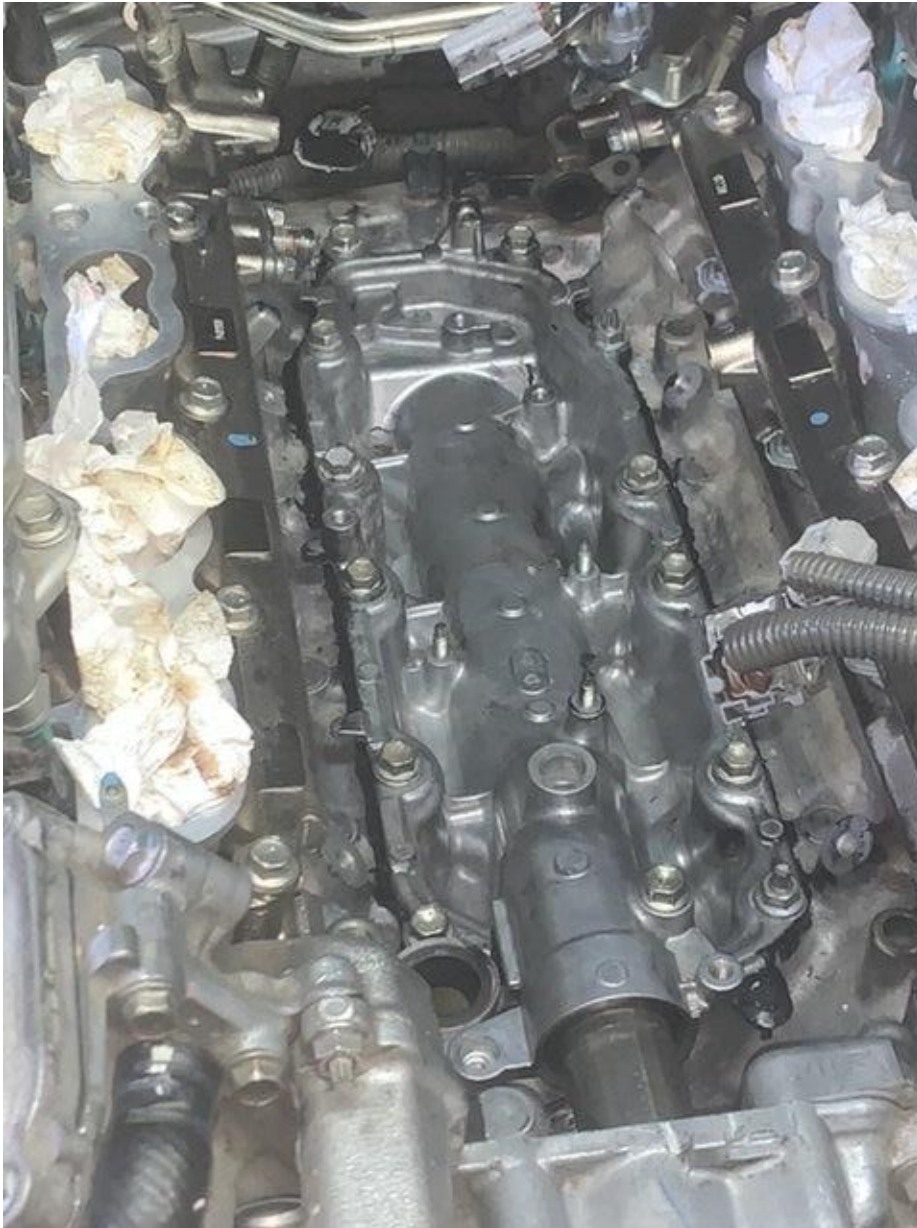
Finished resealed Valley Plate
