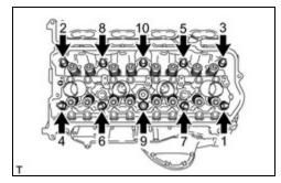
(c) Remove the cylinder head and gasket.
