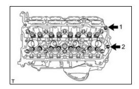
(b) Using a 10 mm bi-hexagon wrench, uniformly loosen the 10 bolts in the sequence shown in the illustration.Remove the 10 cylinder head bolts and plate washers.
