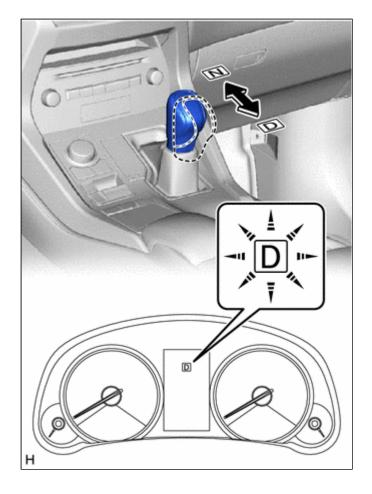
(k) Check that the D shift indicator comes on for 2 seconds.
