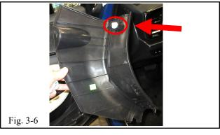
(f) Reattach the one (1) push clip to the cowl trim if necessary (Fig. 3-6).
