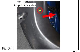
(d) Remove the cowl by pulling rearward and inward to disengage one (1) attachment clip and retain for reassembly (Fig. 5-4).
