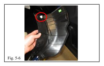
(f) Reattach the one (1) push clip to the cowl trim if necessary (Fig. 5-6).
