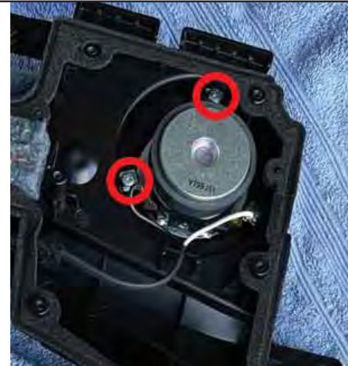
8. Remove three (3) Phillips screws (2 of 3 shown) securing speaker to speaker assembly, disconnect harness and remove speaker.
