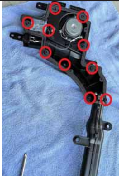
7. Remove ten (10) Phillips screws (circled) securing back panel of speaker assembly, then remove panel.
