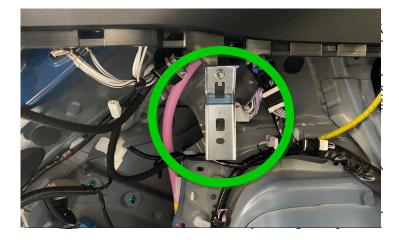
c. Disconnect the driver side combination lamp connectors (Fig. 7-3).
