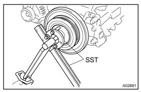
18. TIGHTEN CRANKSHAFT PULLEY BOLT
