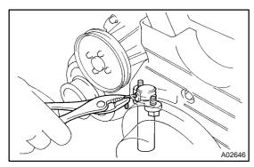
(c) Remove the 1.5 mm hexagon wrench from the tensioner with pliers.
