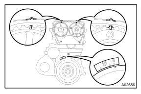
(b) Check that each pulley aligns with the timing marks as shown in the illustration.
