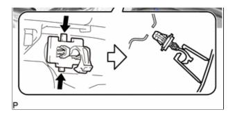
d. Disengage the 3 guides to remove the front pillar garnish LH as shown in the illustration.
