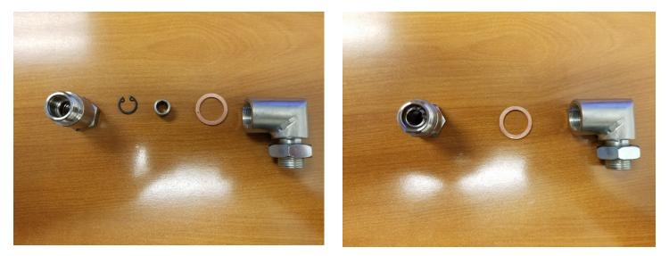
Install restrictor with the larges hole to start. This restrictor works for most applications. If a P0420 (bank1) or P0430 (bank2) code is seen, use the next size smaller hole restrictor. If a slow response or low voltage code is seen, remove the restrictor and run with no restrictor in the extender.
