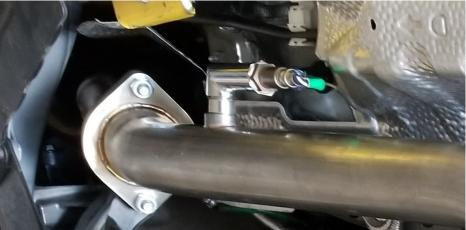
Install on the rear O2 sensors in the midpipe, do not install on the front O2 sensors.
