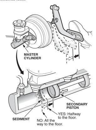
To completely avoid this potential problem, use any of the brake pressure bleeder equipment available through the Acura Tool and Equipment Program (call 888-424-6857). The equipment makes brake bleeding much quicker and easier.
