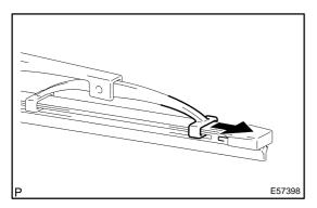
(b) Install the wiper rubber LH so that the head part (larger side) of the wiper rubber faces the arm axle side.NOTICE:
