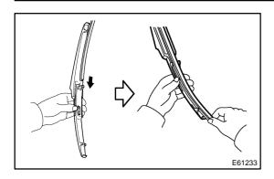
(b) Insert the rear wiper rubber from the claw position of the middle of the rear wiper blade to the end.
