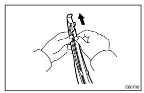
(c) After passing the rear wiper rubber through the rear end side claw, allow it to stick out from the rear end stopper and slide it through the front tip side claw.
