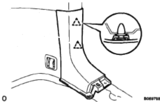
Fig. 19: Identifying Clips On Floor Finish Side Plate Courtesy of TOYOTA MOTOR SALES, U.S.A., INC.
