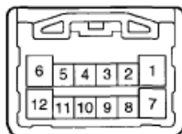
Fig. 8: Identifying Multiplex Network Switch (Front Passenger Side) Connector Terminals Courtesy of TOYOTA MOTOR SALES, U.S.A., INC.
