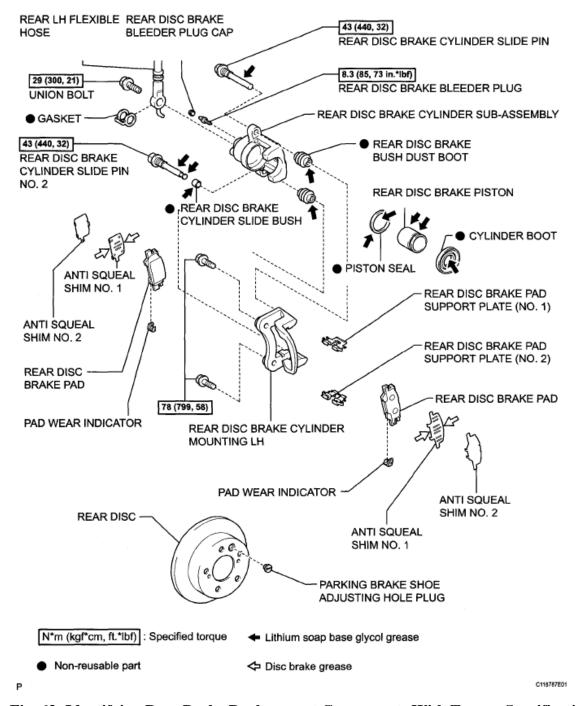
Fig. 63: Identifying Rear Brake Replacement Components With Torque Specifications Courtesy of TOYOTA MOTOR SALES, U.S.A., INC.
