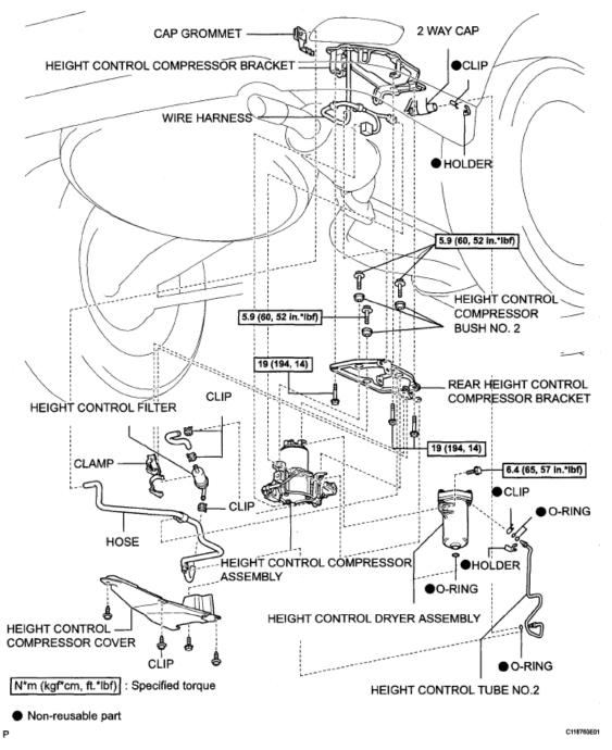
**Fig. 137: Identifying Height Control Compressor Replacement Components With Torque Specifications** Courtesy of TOYOTA MOTOR SALES, U.S.A., INC.
