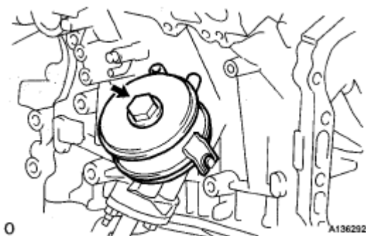
Fig. 466: Identifying Oil Cooler Assembly Union Bolt Courtesy of TOYOTA MOTOR SALES, U.S.A., INC.
