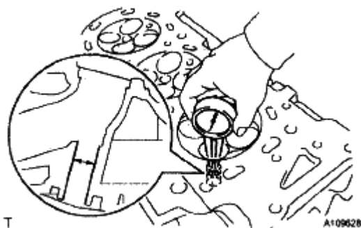
Fig. 372: Measuring Bush Bore Diameter Of Cylinder Head Using Caliper Gauge Courtesy of TOYOTA MOTOR SALES, U.S.A., INC.
