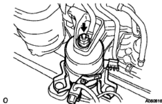
Fig. 71: Identifying Engine Mounting Insulator FR Bolt Courtesy of TOYOTA MOTOR SALES, U.S.A., INC.
