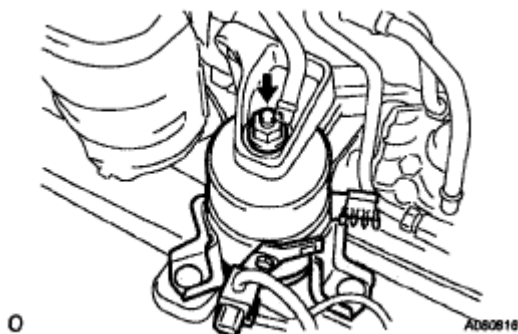
Fig. 122: Identifying Engine Mounting Insulator FR Bolt Courtesy of TOYOTA MOTOR SALES, U.S.A., INC.
