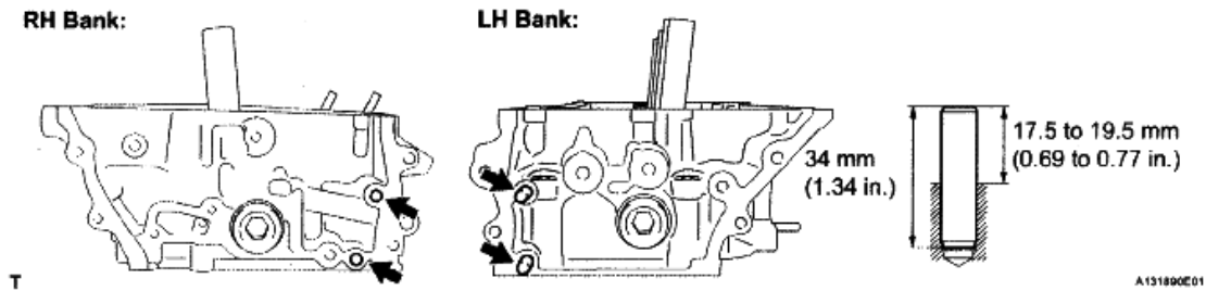
Fig. 379: Identifying Straight Pin Position Courtesy of TOYOTA MOTOR SALES, U.S.A., INC.
