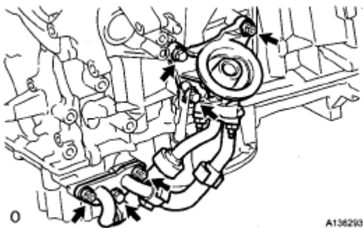
Fig. 185: Identifying No. 1 Oil Cooler Bracket Bolts & Nuts Courtesy of TOYOTA MOTOR SALES, U.S.A., INC.
