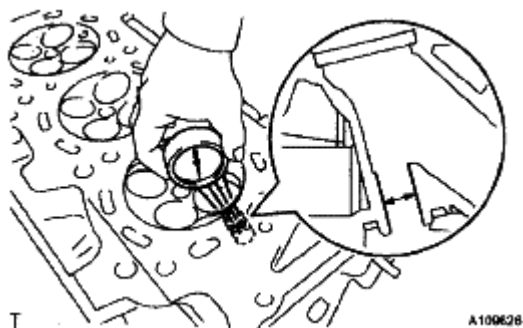
Fig. 369: Measuring Bush Bore Diameter Of Cylinder Head Using Caliper Gauge Courtesy of TOYOTA MOTOR SALES, U.S.A., INC.
