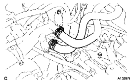
Fig. 141: Identifying Heater Outlet Water Hose Courtesy of TOYOTA MOTOR SALES, U.S.A., INC.
