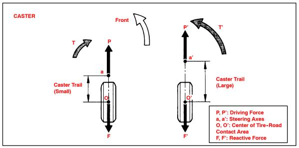
If the cross camber or caster is within the specified range (30' or less), noticeable vehicle pulling will not occur due to side-to-side differences in camber or caster.
