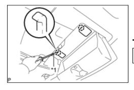
(c) Using a screwdriver wrapped with protective tape, disengage the 2 claws and disconnect the 2 caps.
