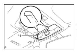
(1) Using a screwdriver wrapped with protective tape, disengage the 2 claws and disconnect the cover.
