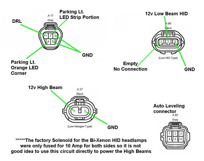
We Actually cut and used Factory DRL connector and wired our own External 40 Amp relay and Fused it at 30 Amps since the factory was 15amp each side.
