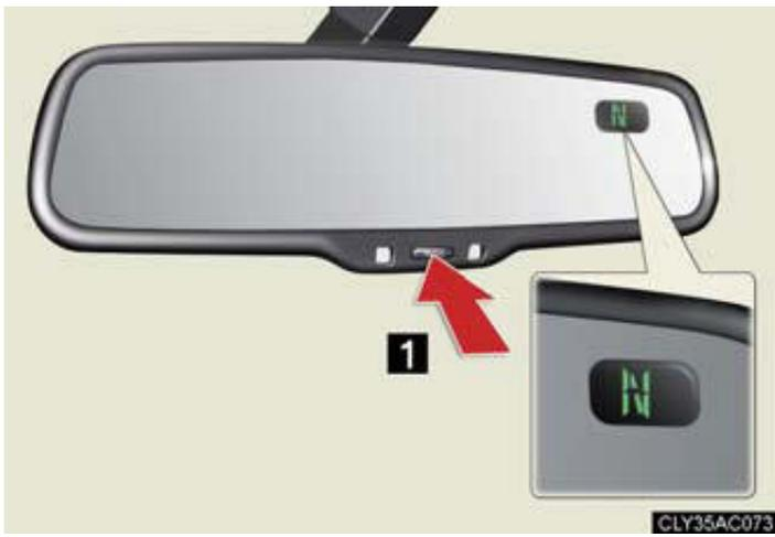
1. To turn the compass on or off, push and hold “AUTO” for 3 seconds.
