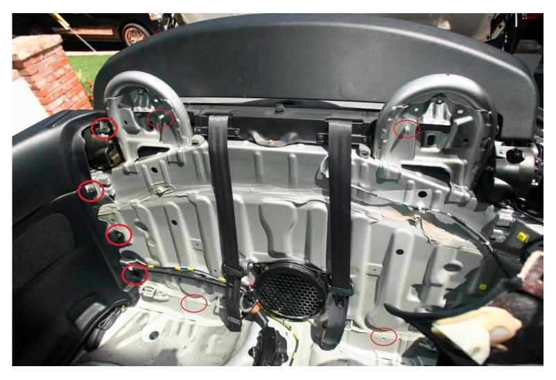
This show the location of the two screw posts under the head rests and two bolt location behind the bottom seat cushion. It also shows the four 10mm screws hidden under the seat back cushion.
