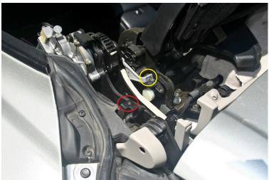
Removing the interior rear quarter panel to access the speakers and window regulator wiring requires the removal of two (2) hidden screws and one retaining clip. In this photo the one screw (red circle) and the clip (yellow circle) have been removed.
