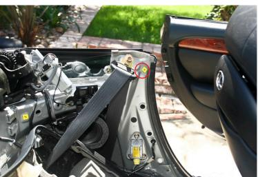
The last hidden screw is behind the seat belt slot in the panel. The slot garnish has four retaining claws two top and two on the bottom along with one guide. Carefully using a taped pry tool you can release the claw and gain access to the screw.
