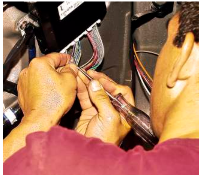
testing for the correct wires by operating the circuit
