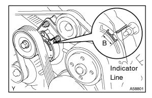
(d) After a new belt has been installed, check that the indicator line is within the B range.
