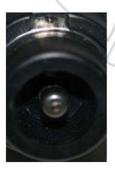
**Fake 2:** Small solder at the top is almost non-existent, protrusion on the center metal post is poorly formed and very small.
