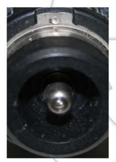
**Fake 1:** Small solder at the top is not centered and poorly formed, protrusion on the center metal post is poor formed and much too small.
