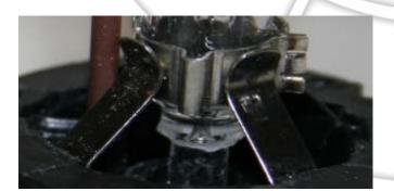
**Fake 2**: Rivets are almost not noticeable, poorly formed lower glass tube, has Zig-Zag lower power wire.
