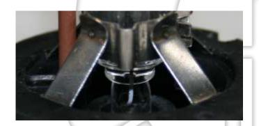
**Fake 1**: Smaller rivets, the glass is nicely formed but the tube is overly large, lower power wire is mostly straight.
