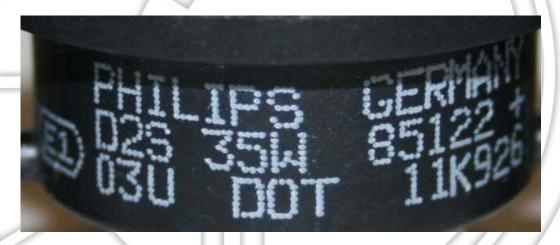
**Fake 1:** Typing still using individual dots but dots blend together, much too bright white, spacing is not uniform between letters and much too narrow between lines.
