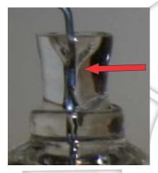
**Real:** Very good formation of the glass, small indentation in the center, return wire wild is encased in glass, bulb is sealed far from the glass body.
