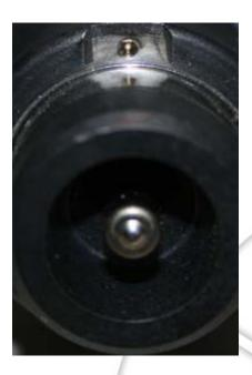
**Real:** Small solder at the top is perfectly centered and nicely formed, protrusion on the center metal post fill most of the surface and nicely formed
