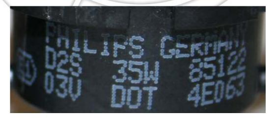
**Fake 2**: Typing still using dots but blend together badly, much too dull white, spacing is not uniform and letters are not formed correctly
