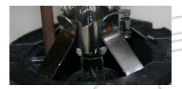
**Real**: Larger perfectly symmetrical rivets, nicely tapered and formed lower glass tube, Zig-Zag Pattern of lower power wire within lower glass.
