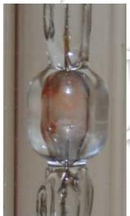
**Fake 1:** Poorly formed capsule more square in shape, poorly formed glass that encases diodes very uneven, salts are red in color which is not correct for an 85122+.
