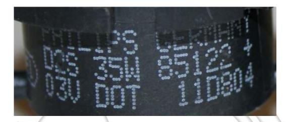
**Real:** Typing is made up of individual dots, matte white in color, spacing between words, letters and lines is all uniform.
