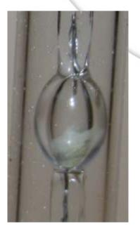
**Fake 2:** Oval shaped capsule that is very small and not symmetrical in shape, thin glass encasing diodes, salts are white and slightly yellow.
