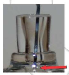
**Fake 1:** Much taller than the real Philips, return wire weld is not encased in the glass, bulb is sealed much closer to center of bulb body.
