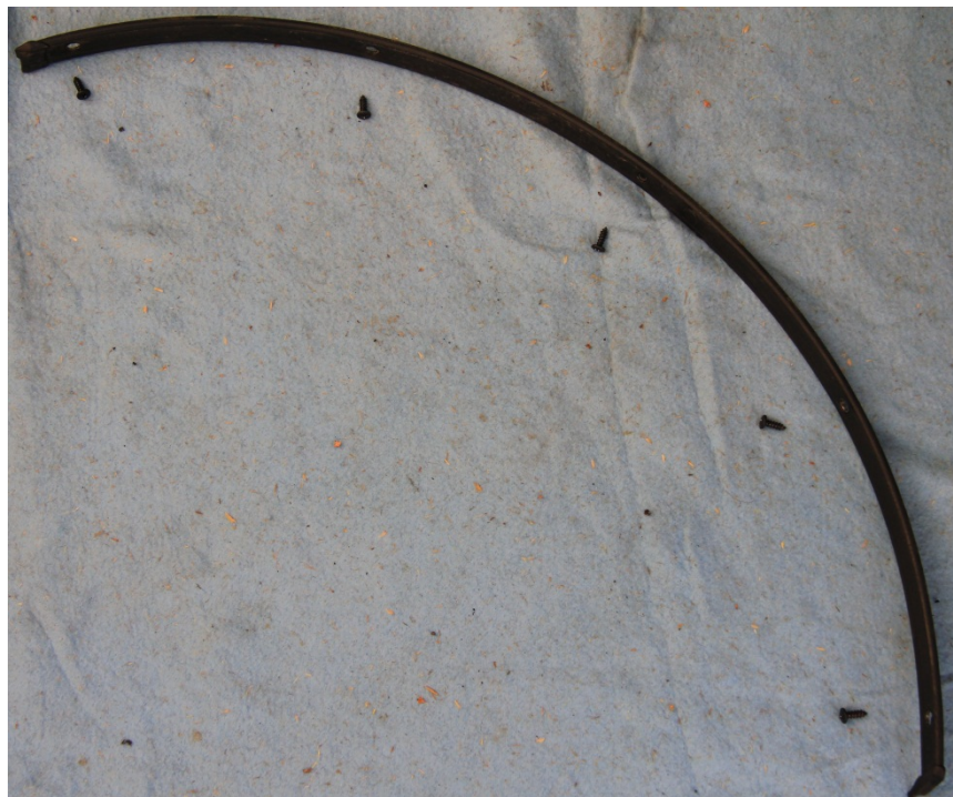
This is what the metal “Wheel Arch Liner Cover” looks like when removed (and laid on a no longer clean picnic blanket!)
