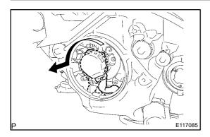
(c) Turn the bulb socket cover in the direction of the arrow and pull it out toward the rear of the vehicle.
