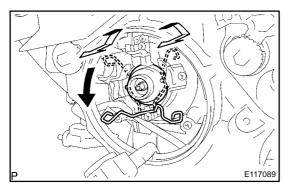
(d) Release the lock of the set spring as shown in the illustration and remove the bulb.
