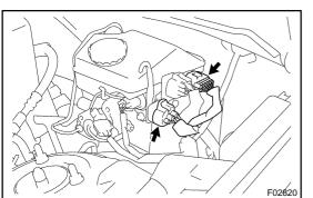
(b) Connect the actuator checker (SST) to the hydraulic brake booster side wire harness via the sub-wire harness S (SST), as shown in the chart below.
